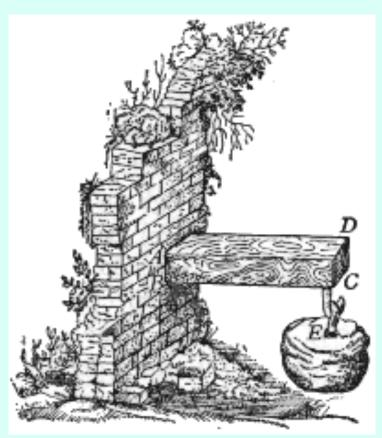
Galileo's illustration of bending test, "Two New Sciences"
